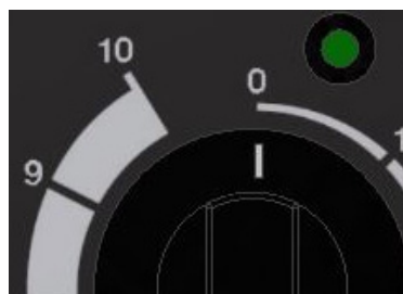
Fig. 0-19 Betjening i Stilling "0" = Afbrudt
